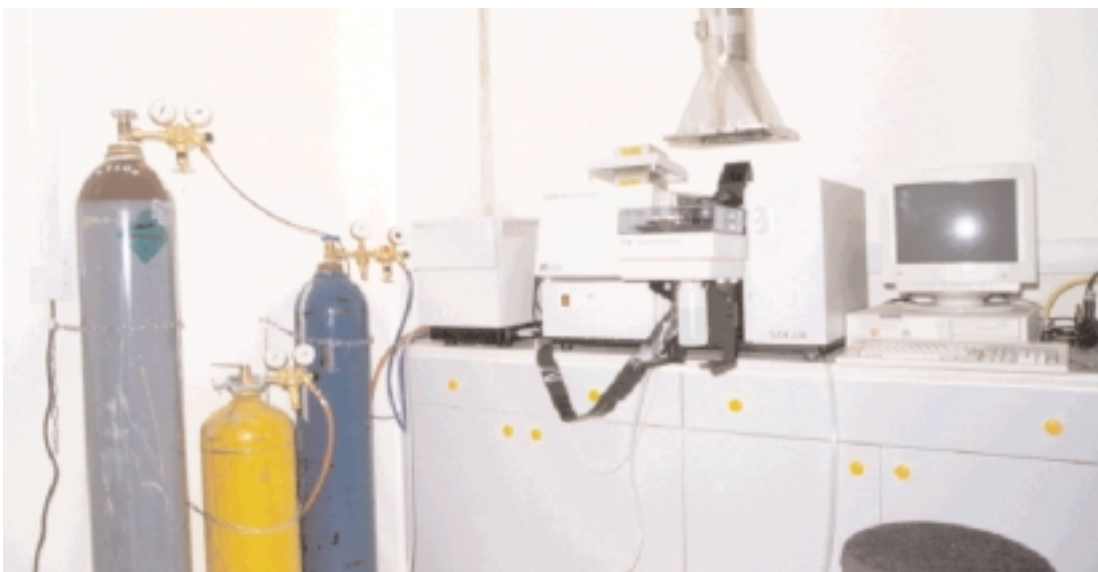
Atomic absorption spectrometer for metals determination
